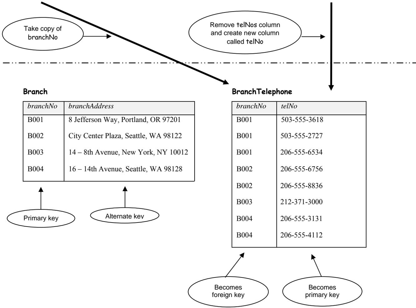
(Note: There is an alternative approach to altering the original Branch table – columns can be added to the original Branch table to hold the individual values for each telephone number, e.g. telNo1, telNo2 and telNo3.)
