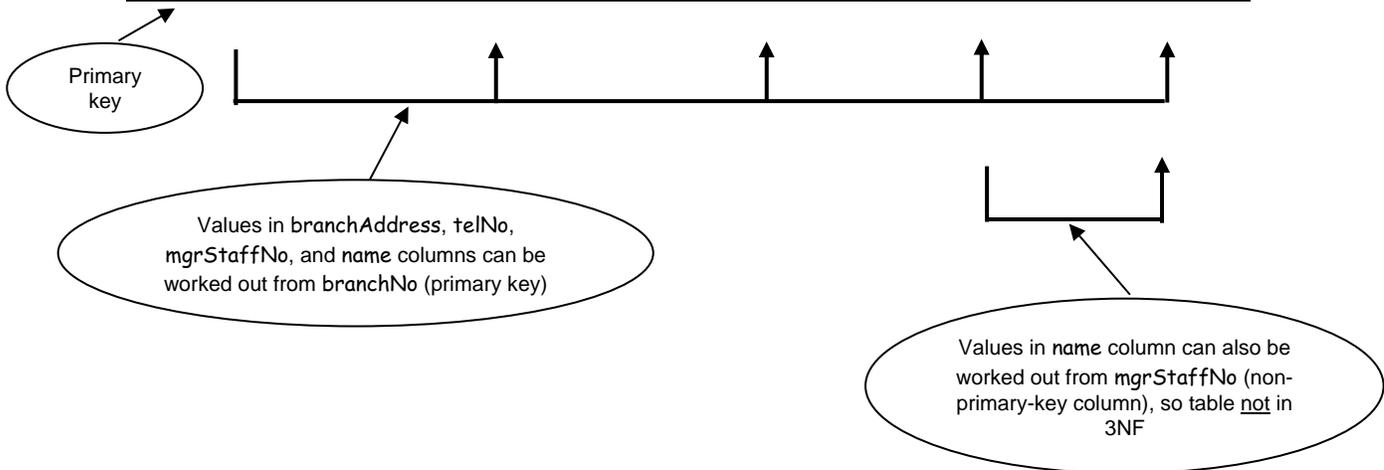
Using Dependency Diagram, it can be represented as shown in the following Figure:
